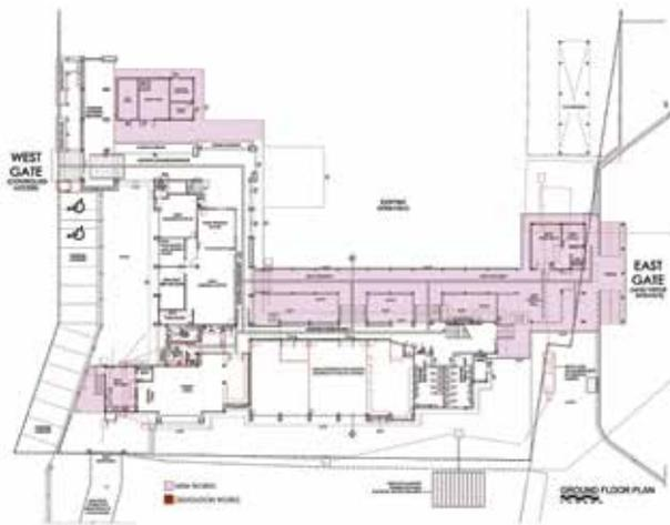
Working within a tight budget to realise the initial Gensler's Masterplan intention, Atelier Timur re-orientated the existing site plan and created a new access to face the main road (Jalan Peninsula) to improve legibility and prominence. Named the East Gate, this portion houses the main public car park, visitor foyer with the customer service counter and Park-shop.
